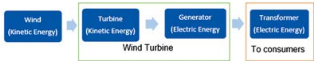
Figure 2: Schematic showing basic energy conversion steps and the respective components involved in harnessing wind energy.
