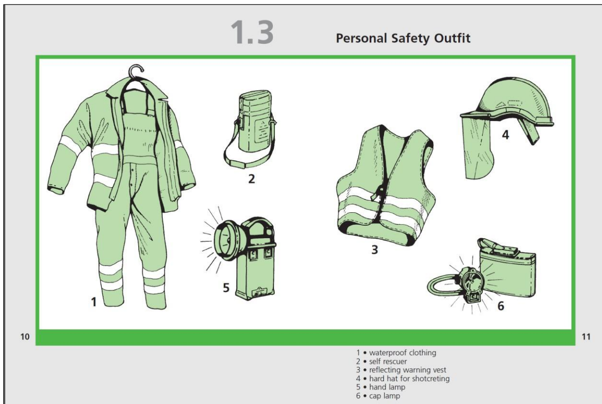
Fig.10 Showing the Personal Safety Outfit for the Team of Tunnelling Work
